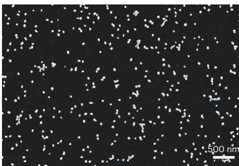
Fig. 6 | SEM image of SHINs on Au single-crystal surface. Approximately 20% coverage of SHINs on single-crystal surface.
