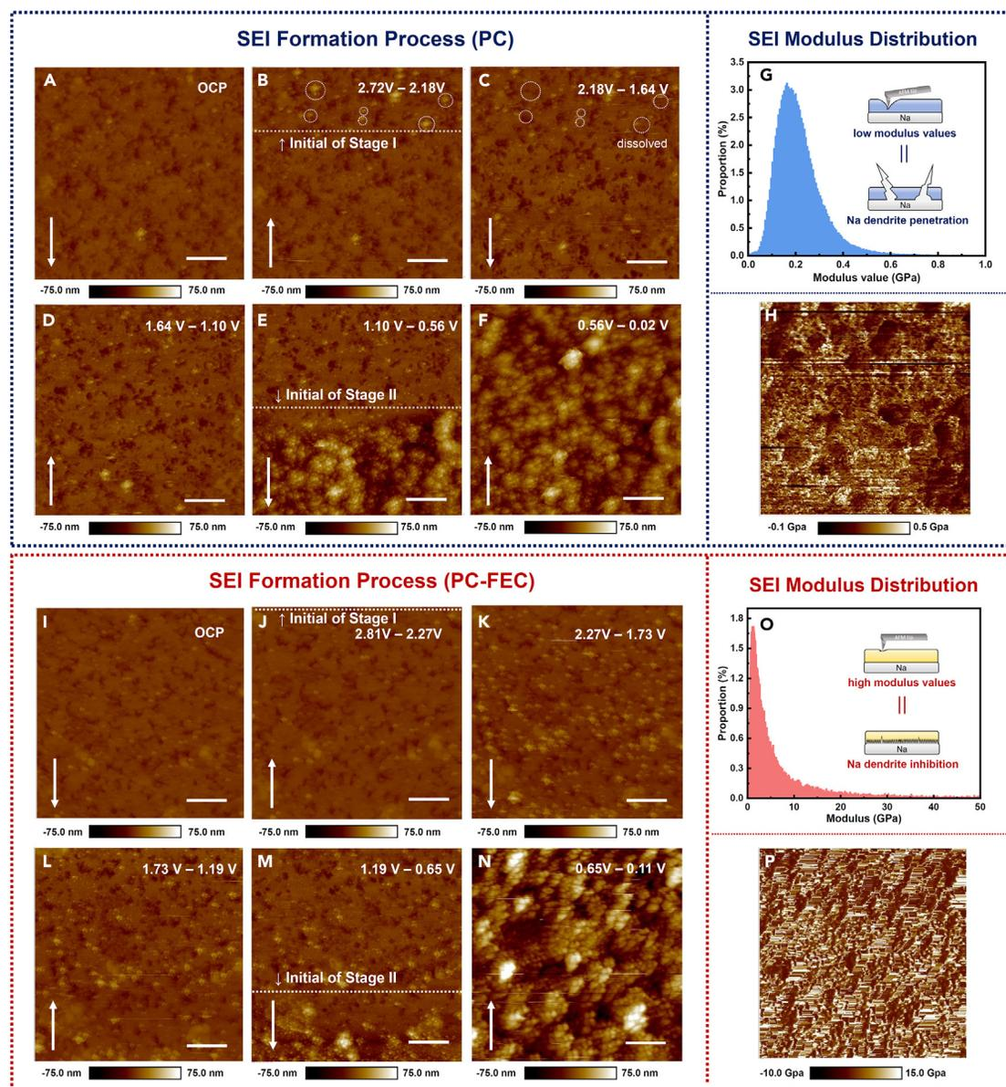
**Figure 2.** *In situ* morphological and mechanical detection of SEI formation process via *in situ* AFM
