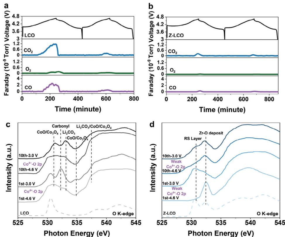
**Figure 3.** Characterizations of LCO/electrolyte interface side reaction during the initial few cycles. The in situ DEMS tests of a) LCO and b) Z-LCO within a voltage range of 3–4.6 V. O K-edge spectra of TEY mode from sXAS measurements of c) LCO and d) Z-LCO during 1<sup>st</sup> and 10<sup>th</sup> cycle within a voltage range of 3–4.6 V.
