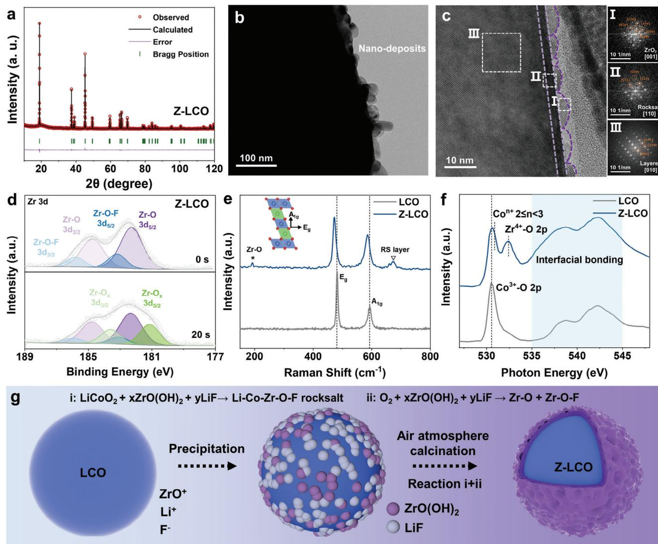
**Figure 1.** Structural characterizations of Z-LCO. a) XRD and Rietveld refinement pattern of Z-LCO. b) HRTEM image of Z-LCO (entire particles without FIB milling treatment). c) HRTEM image and corresponding fast Fourier transform (FFT) results of Z-LCO after FIB milling treatment. d) The Zr 3d XPS patterns of Z-LCO. e) The Raman spectra of LCO and Z-LCO. f) O K-edge spectra of TEY mode from sXAS measurements of LCO and Z-LCO. g) The schematic diagram of synthesis process for Z-LCO.
