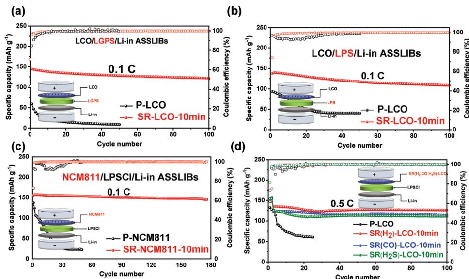
**Figure 6.** Generality and transferability. a,b) The cycling performance of all-solid-state lithium-ion batteries (ASSLBs) with pristine LCO (P-LCO) and SR-LCO-10 min using LGPS and LPS solid-electrolytes (SEs), respectively. c) The cycling performance of ASSLBs with NCM811 before and after gas–solid interface reduction reaction (GSIRR) process. d) The cycling performance of ASSLBs with LCO before and after treatment by various reducing gases ( $H_2$ , CO, and  $H_2S$ ) at 0.5 C.
