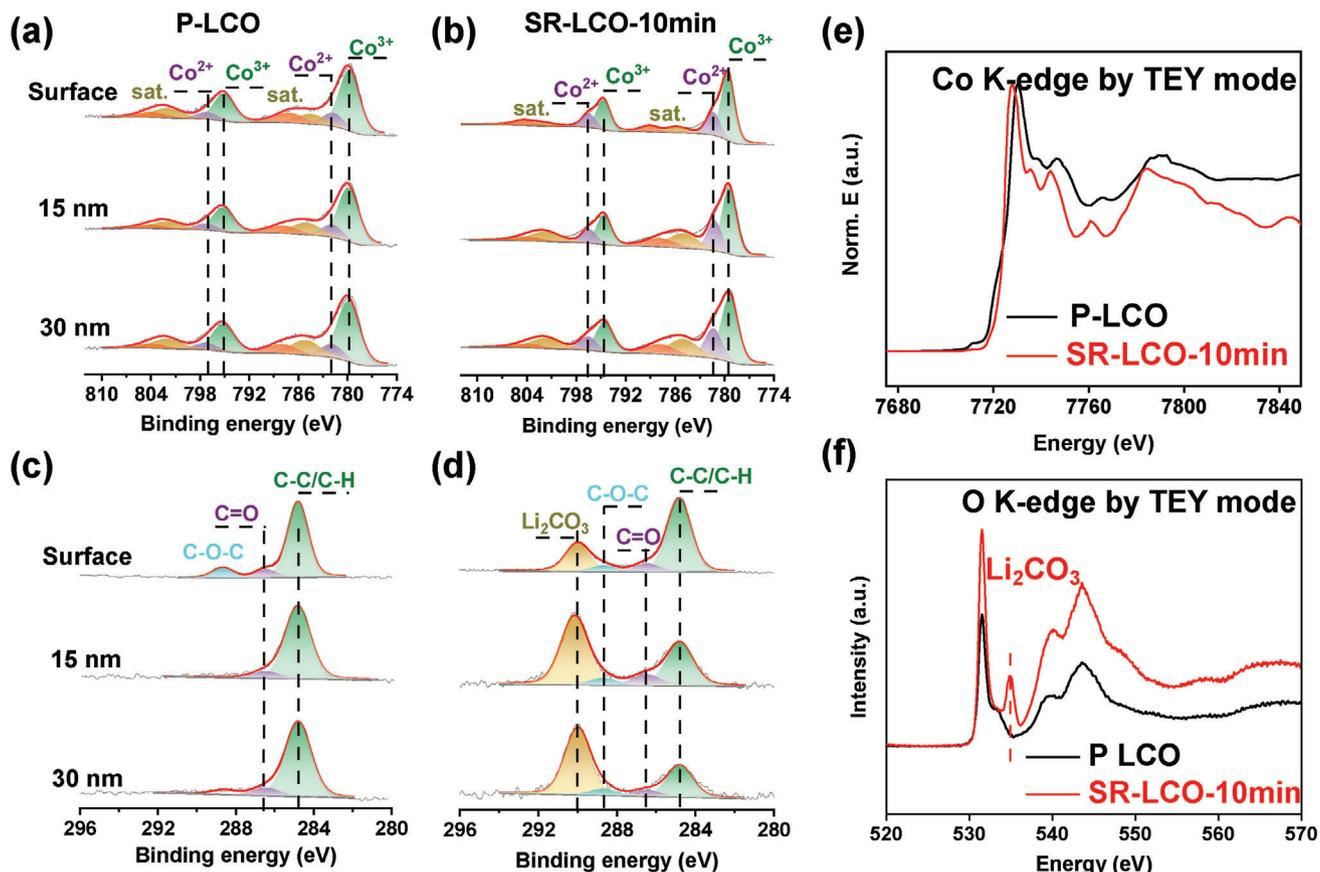
**Figure 2.** Surface characterizations of X-ray photoelectron spectroscopy (XPS) and X-ray absorption spectroscopy (XAS). a–d) XPS spectra of Co and C for the pristine LCO (P-LCO) and SR-LCO-10 min samples at different depths. e, f) XAS of P-LCO and SR-LCO-10 min: Co K-edge in total electron yield (TEY) mode and O K-edge in TEY mode, respectively.
