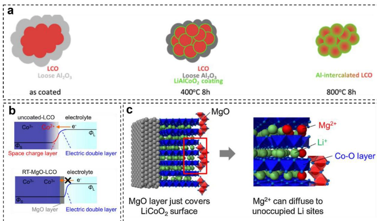
Fig. 6. (a) Schematic diagram of the interaction between  $\text{Al}_2\text{O}_3$  and LCO. Reproduced with permission [58]. Copyright 2017, ACS. (b) Schematic diagram illustrating the effect of MgO coating on LCO surface. Reproduced with permission [57]. Copyright 2014, ECSJ. (c) Schematic diagram illustrating the supporting role of  $\text{Mg}^{2+}$  occupying Li sites [57]. Copyright 2014, ECSJ.
