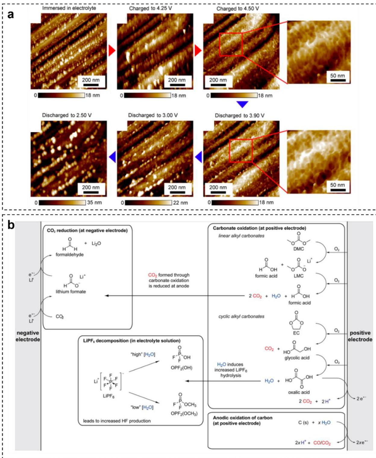
Fig. 4. (a) AFM images of in-situ monitoring of the CEI film formation and decomposition on the edge plane of LiCoO<sub>2</sub> crystal. Reproduced with permission [40]. Copyright 2017, ACS. (b) The electrolyte decomposition reactions that occur at high voltages (or high SOC) initiated at the positive electrode. Reproduced with permission [41]. Copyright 2020, ACS.
