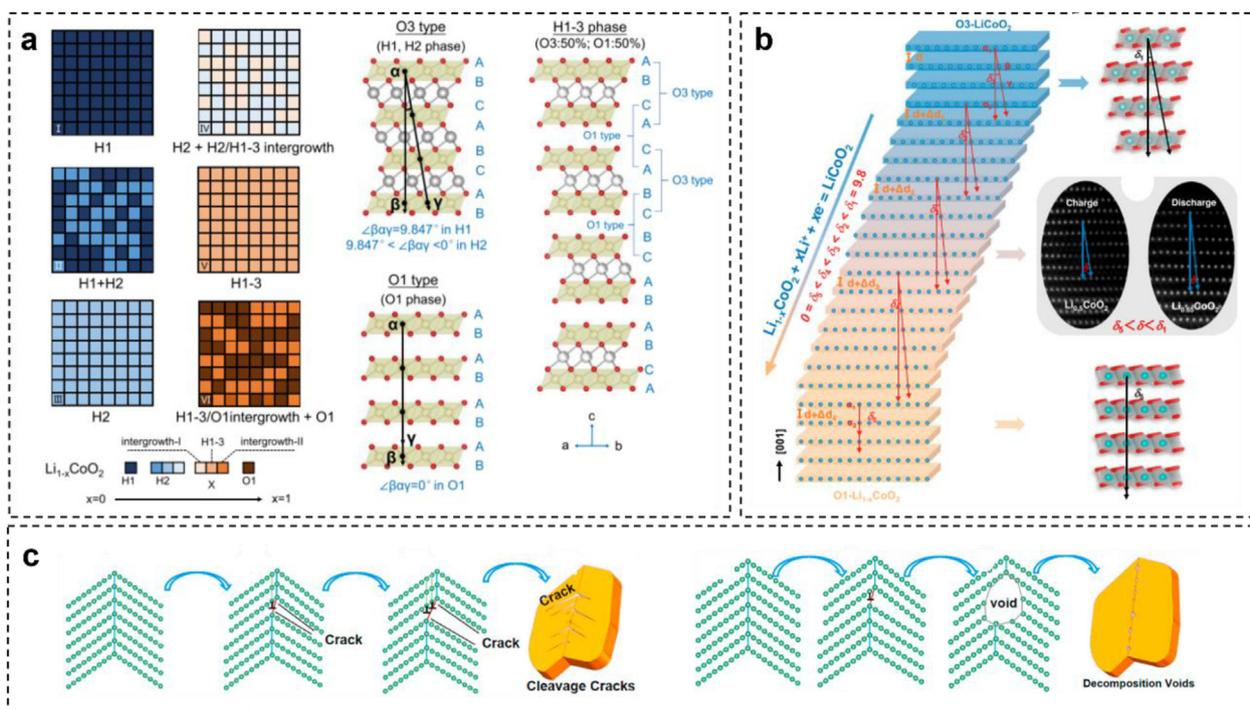
Fig. 1. (a) Diagram of LCO structure distribution during the entire phase transition process. Reproduced with permission [20]. Copyright 2023, ACS. (b) Collective glide of  $\text{CoO}_6$  slabs in  $\text{Li}_{1-x}\text{CoO}_2$ . Reproduced with permission [21]. Copyright 2022, PNAS. (c) Nucleation and propagation of cleavage cracks and decomposition cracks. Reproduced with permission [25]. Copyright 2020, Elsevier.
